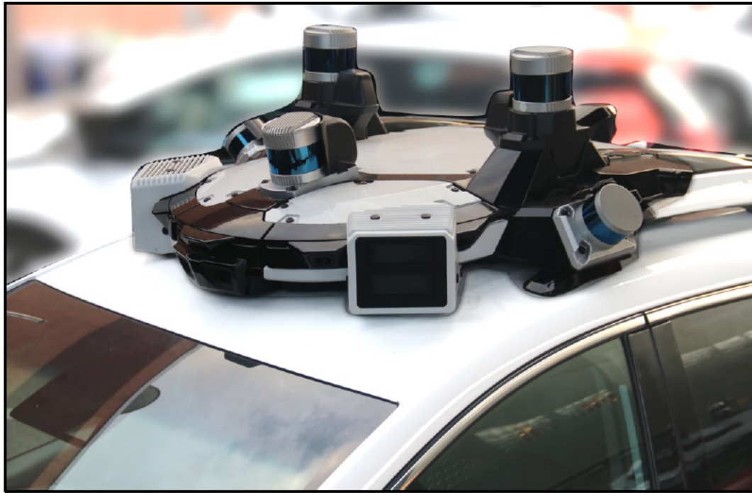
Figure 7. Roof mounted sensor array which includes lidars, cameras, and radars.
